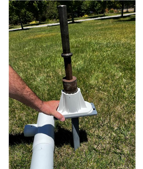
Check to ensure the pin at the back of the boot is secure. This holds the boot in place to the ground plate.
