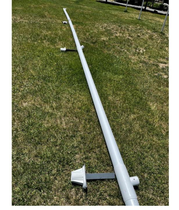
Install the ground plate with the Barriers tool using a hydraulic jack hammer. The boot remains attached to the ground plate.
